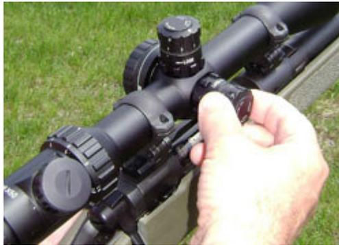
*The most precise windage compensation results from target knobs, such as this 1/8th Minute-of-Angle knob on a Millett TRS scope. The Millett LRS has a 1/4 MOA knob.*
